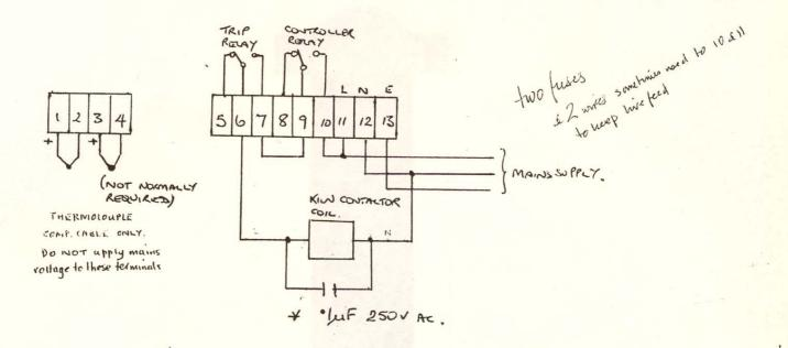
\* A CAPACITOR MUST BE CONNECTED ACROSS ALL INDUCTIVE LOADS AS
