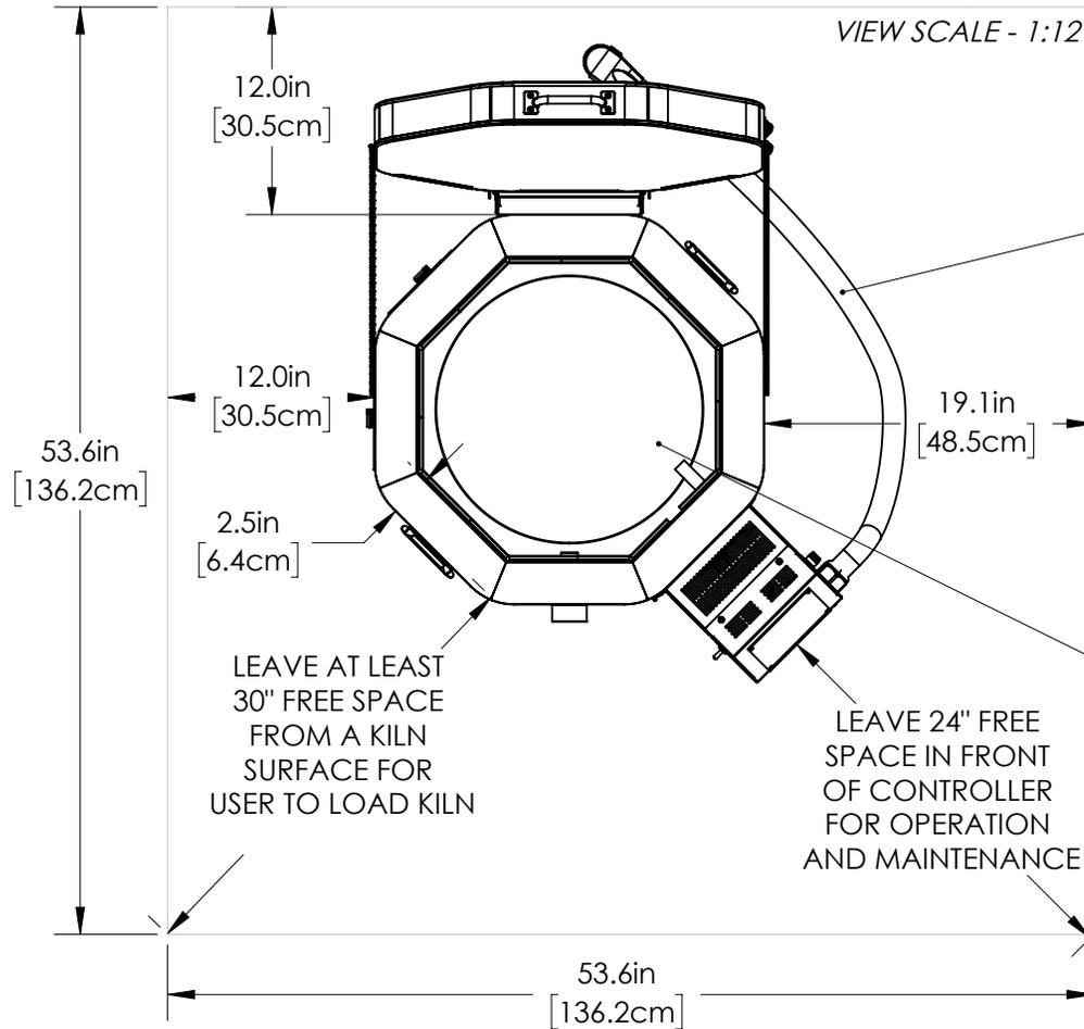
POWER CORD IS 6 FEET LONG: NEMA 6-50 FOR SINGLE PHASE OR 15-50 FOR THREE PHASE. ALTERNATELY KILN MAY BE HARD WIRED TO A FUSED DISCONNECT BOX. ALSO 6-30 AND 10-30 CORDS ARE AVAILABLE AS AN OPTION.
