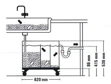
The TA is placed on a metal trolley and can be moved for cleaning after unscrewing the siphon and removing the inlet pipe (attention: please only pull down on the trolley and not upwards)!
