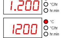
If the left-hand decimal point in the display is lit then the Firemaster is locked. Press and hold in both the ♠ & ♣ keys for 5 seconds to unlock the Firemaster.
