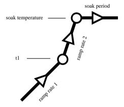
A Firemaster firing segment comprises 2 ramps followed by a soak period. A single segment can be used for simple firing (biscuit firing for example) or up to 9 segments can be used per program for complex firing (crystal glazing or glass-making for example).
