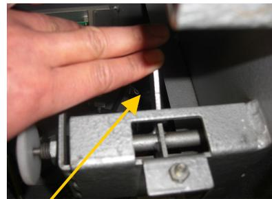
Move the pedal or lever up and down to ensure parts are fully lubricated with the WD-40
