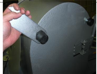
Remove the four feet off of the bottom of the wheel and remove the metal cover.
