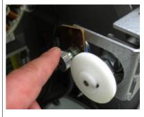
5.Turn the potentiometer until the wheel head starts to turn, then turn it the opposite way until the wheel head stops.
