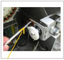
6.Screw down the new potentiometer in place.
