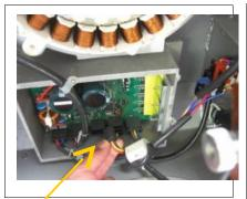
assembly from the control board by squeezing the sides of the clip and pulling.
