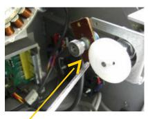
3. Unscrew the two screws then install new potentiometer
