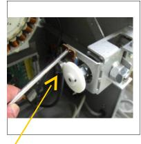
6. When the wheel head stops, slide the potentiometer up against the white gear and tighten the screws down. Then replace the cover 4 feet. Your wheel should now be running from stop to 250 rpm.
