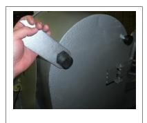
1.Remove the four feet off of the bottom of the wheel and remove the metal cover.
