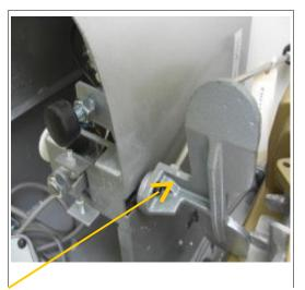
**6.**Make sure the pedal is in the stop position and the power is on
