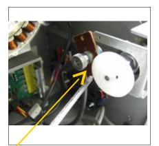
4. Move the potentiometer (silver gear) away from the white plastic gear so they are not touching
