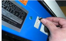
Make sure the pedal is in the stop position and the power is on
