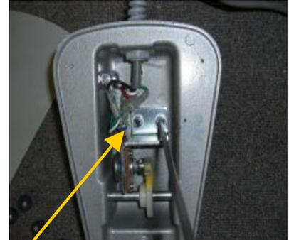
3. Loosen the two screws connecting the potentiometer bracket to the foot pedal housing
