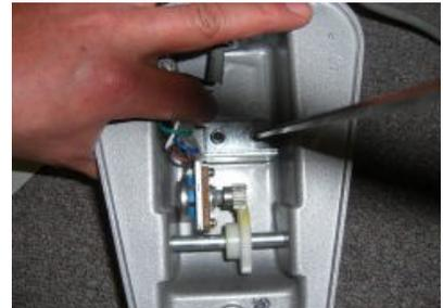
6. When the wheel head stops, slide the potentiometer up against the white gear and tighten the screws that hold the bracket back down. Then replace the cover and 4 feet. Your wheel should now be running from stop to 250 rpm.
