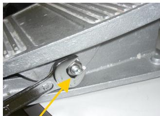
Then loosen the inner bolt until
