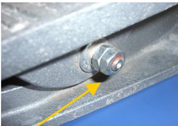
Loosen the outer bolt first,
