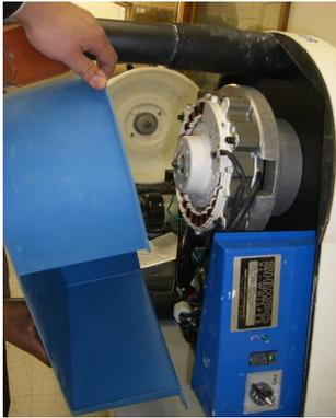
1.Remove undercover by removing all undercover screws then sliding the undercover off.
