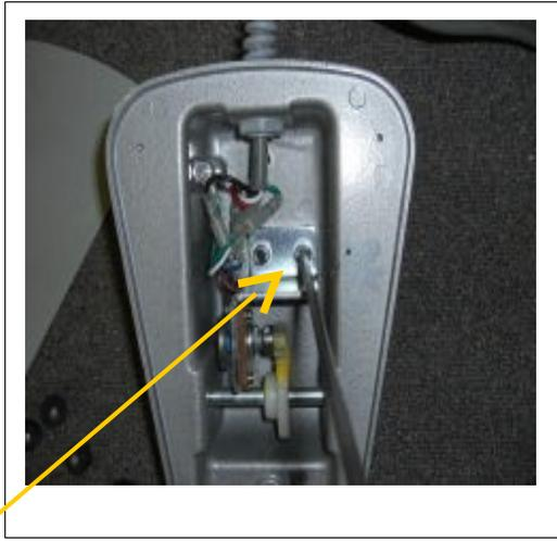
**6. Loosen the two screws connecting the potentiometer bracket to the foot pedal housing**
