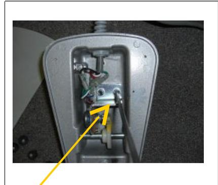
**3.Unscrew the two bolts potentiometer bracket to the foot pedal housing**
