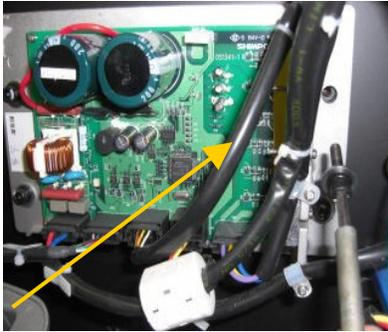
**7. Then install the new controller and remember to clip on all wire harnesses and re-attach the ground wire**
