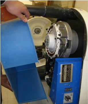
1.Remove the undercover by removing all undercover screws then sliding the undercover off.
