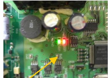
**9. Control board should be flashing both lights:
