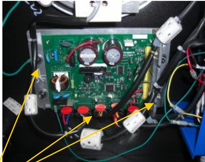
**11. Make sure that all parts are back in place, all wire harnesses are securely clipped in, ground wire is fastened, and controller is firmly screwed on. Then replace blue undercover.**
