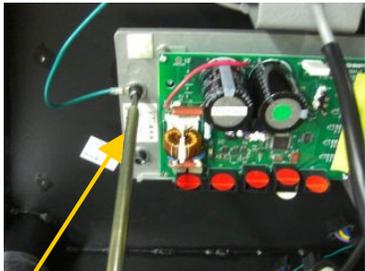
6.Unscrew the 4 bolts including the green ground wire to take off the controller
