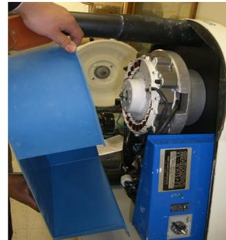
Place the wheel vertical and remove the undercover by removing all undercover screws then sliding the undercover off.
