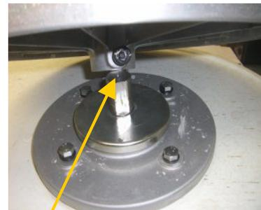
The wheel head bolt must be tightened onto the flat part of the shaft. If it is not on properly, the shaft will spin but the wheel head will not have any torque.
