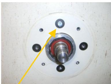
Place the first bolt back in and tighten. Then lean the wheel to a vertical position again. Replace all parts in the same way they were taken off.
