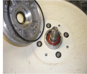
Remove the bearing cover and rubber ring
