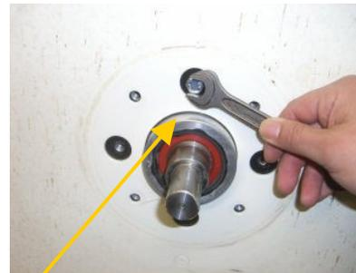
Lean the wheel upside down and support it so that the shaft does not touch the ground. Take off the last bolt by supporting motor from the other side
