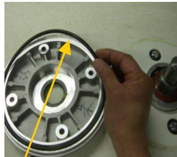
Make sure you re-install the rubber ring. This will insure no water will leak into the bearings.
