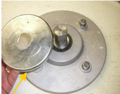
Remove the metal cover from the shaft that fits over the bearing plate
