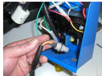
Remove the potentiometer harness from the inside of the blue panel
