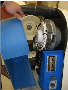
Remove the undercover by removing all undercover screws then sliding the undercover off.
