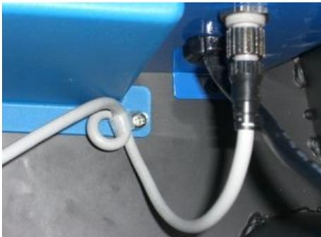
**ATTACH A ZIP TIE TO THE OUTSIDE OF THE BLUE PANEL SECURING THE FOOT PEDAL CORD**
