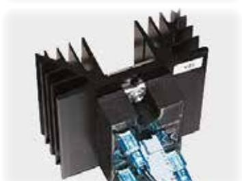
Solid state relays ensure low-noise heater operation
