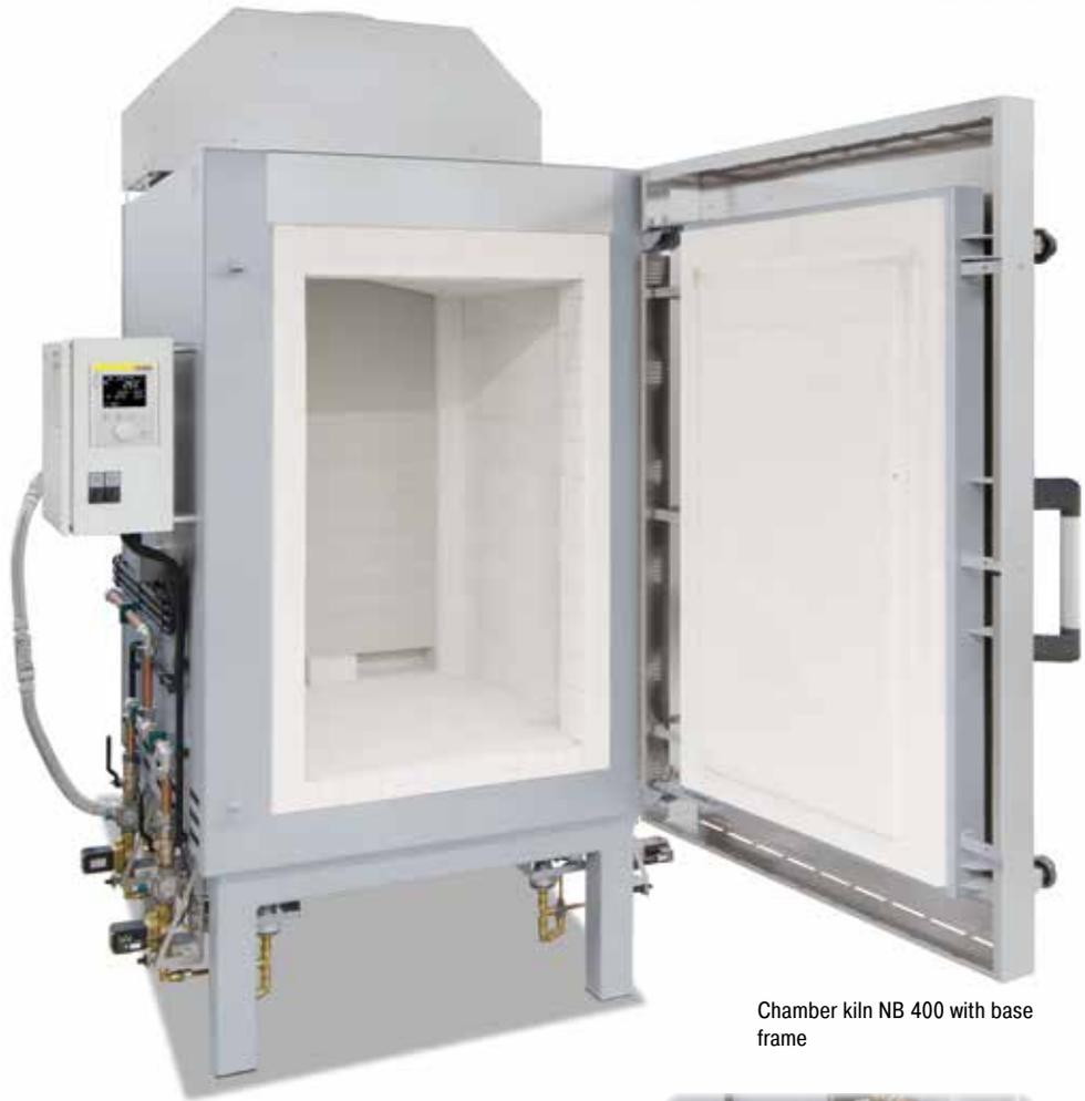
Chamber kiln NB 400 with base frame
