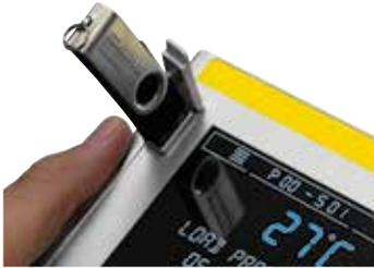
The process documentation with NTLog Basic requires no additional thermocouples or sensors. Only data recorded which are available in the controller. The data stored on the USB stick (up to 80,000 data records, format CSV) can afterwards be evaluated on the PC either via NTGraph or a spreadsheet software used by the customer (e.g. MS-Excel). For protection against data manipulation the generated data records contain checksums.
