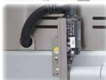
Heating switches off when the lid is opened
