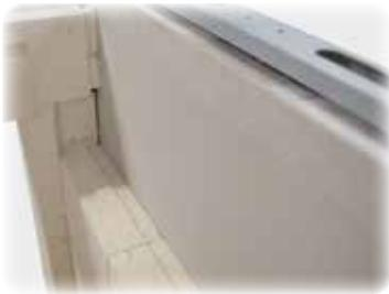
Multi-layer insulation with light-weight refractory bricks and energy-saving backing insulation adapted to the maximum kiln temperature
