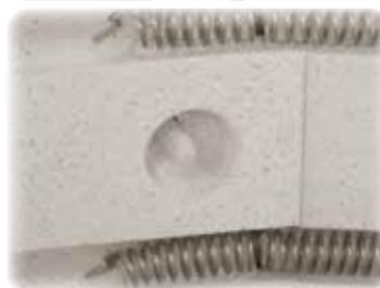
Thermocouple protected in the insulation
