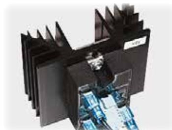
Solid state relays ensure low noise heater operation
