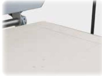
Level table surface with rugged refractory insulation and marked charge surface
