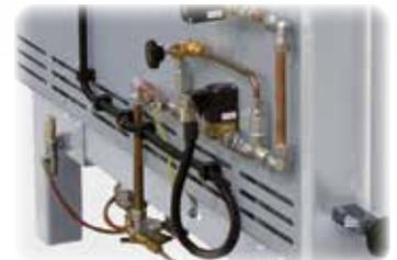
Gas lines and thermocouple at the chamber kiln
