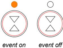
While programming either a ramp rate or a soak time the event output can be switched on or off by pressing the event key. The event output will be ON when the event lamp is on. The event output will be OFF when the event lamp is off. The event lamp also shows the status of the event output when the controller is running a program.
