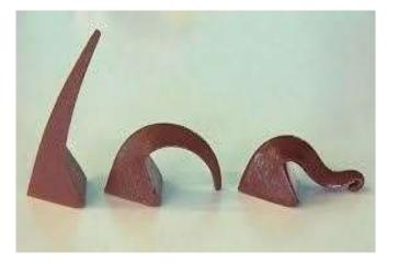
The above illustration shows the three cone system, the cone on the left is the guard cone, one cone above the target cone which is the centre cone, on the right is the guide cone. The target cone is perfectly fired, the guide cone is over-fired and the guard cone is underfired.
