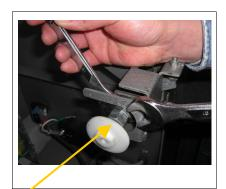
Loosen the first bolt (double nut)
