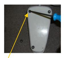
1.Unscrew the 4 feet using the Phillips screwdriver
