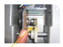
4. Move the potentiometer (silver gear) away from the white plastic gear so they are not touching
