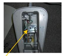
3.Loosen the two screws connecting the potentiometer bracket to the foot pedal housing
