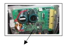
2) Turn the wheel off and then on again while watching the control board. If the controller is in good conditions, you should see lights (red and green, then green blinking). If there are no lights on the control board, you have a bad board. Please notify Shimpo your need to order one and have your wheel's serial number ready.
