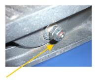
Loosen the outer bolt first, then the inner bolt
