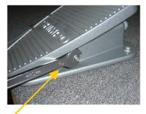
Adjust the U-nut to change the tension of the foot pedal.
