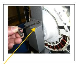
1.Remove undercover by removing all undercover screws then sliding the undercover off.
