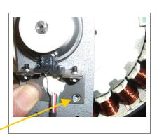
6. Squeeze and unclip/ unplug the encoder reader harness from the circuit board.
