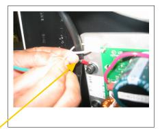
9. Futher secure the wire to the wire holder located on the circuit board holder with a zip tie.
