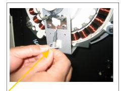
8. Secure the encoder reader wire to the wire holder with a zip tie.
