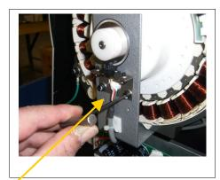
3. Carefully remove the two encoder reader bolts.
