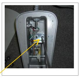
6.Loosen the two screws connecting the potentiometer bracket to the foot pedal housing
