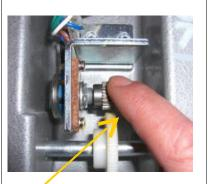
5. Turn the potentiometer until the wheel head starts to turn, then turn it the opposite way until the wheel head stops.
