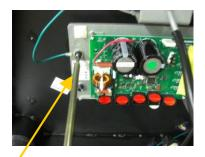
6.Unscrew the 4 bolts including the green ground wire to take off the controller
