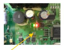
9. Control board should be flashing both lights: LED1=Green LED2 =RED
