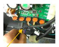
5.Un-clip all 5 cables from the control board by squeezing the sides of the clip and pulling
