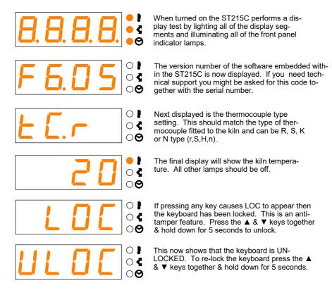
If any mimic panel lamps are on then the ST215C is firing. To stop the firing press the  $\blacktriangleright \blacksquare$  key.
