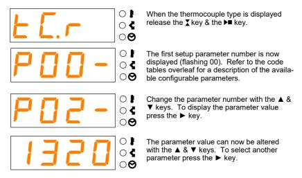
Pressing both the X key & the ▶■ key at any time causes the configuration parameters to be stored. The instrument will then reboot.
