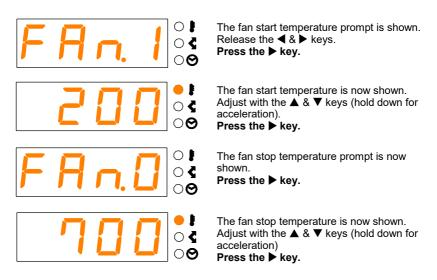
The ST215C will now reset and the new fan control temperatures will be stored.
