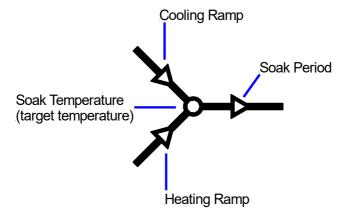
An ST215C firing segment comprises a ramp followed by a soak period. Two segments can be used for simple firing (biscuit firing for example) or several segments can be used per program for complex firing (crystal glazing or glass-making for example).
