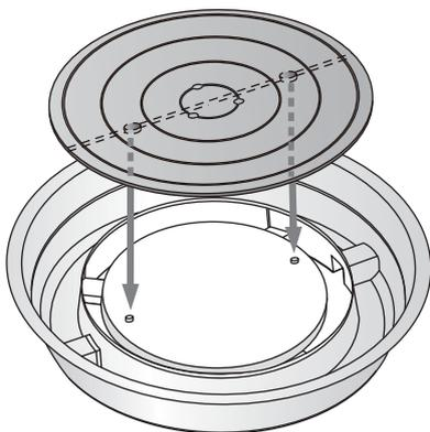
① Install pins adjusting the position.
